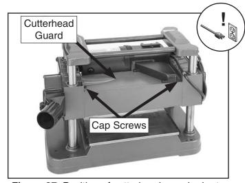
**Figure 27.** Position of cutterhead guard prior to disassembly.
